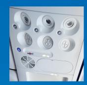
Ceiling Panels/Ducts/ Passenger Service Units (PSU)
